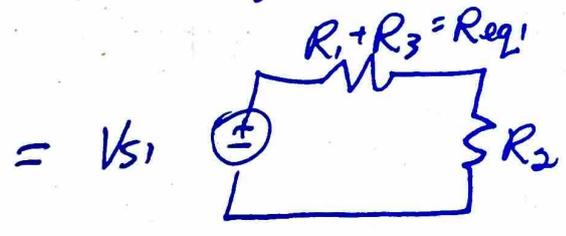
$$\text{Then } V_{R_2} = V_1 \left( \frac{R_2}{R_1 + R_3 + R_2} \right)$$
