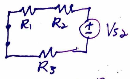
$$V_{R_2} = V_2 \left( \frac{R_2}{R_1 + R_2 + R_3} \right)$$
