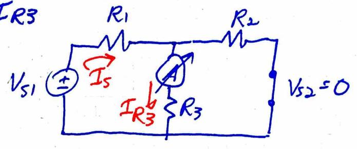
$$R_{eq} = R_1 + R_2 \parallel R_3$$
